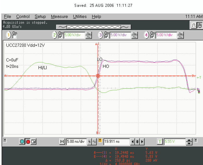
Figure 33. 20-ns Input Pulse Delay Matching
