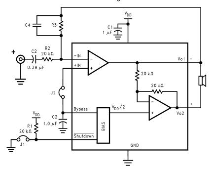
Figure 68. HIGHER GAIN AUDIO AMPLIFIER
