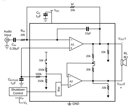
Figure 7. Typical Audio Amplifier Application Circuit
