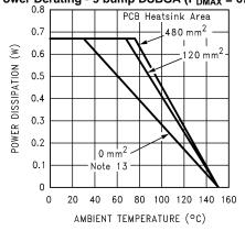
Note:  $(P_{DMAX} = 670 \text{mW for 5V}, 8\Omega)$
