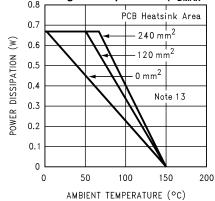
Note:  $(P_{DMAX} = 670mW \text{ for 5V}, 8\Omega)$ Figure 41. Ambient Temperature in Degrees C
