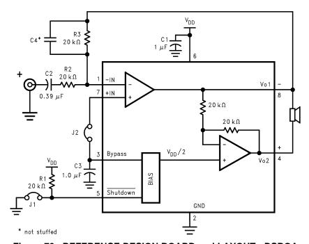
Figure 70. REFERENCE DESIGN BOARD and LAYOUT - DSBGA
