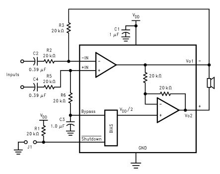
Figure 69. DIFFERENTIAL AMPLIFIER CONFIGURATION FOR LM4890
