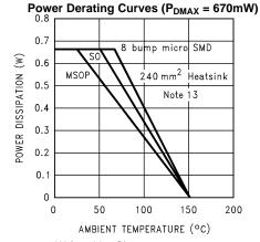
Note:  $(P_{DMAX} = 670 mW \text{ for 5V}, 8\Omega)$ Figure 40. Ambient Temperature in Degrees C
