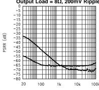
FREQUENCY (Hz) Figure 39. LM4890 = Bottom Trace LM4877 = Top Trace
