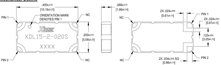
Dimensions are in Inches [Millimeters] XDL15-2-020S Mechanical Outline
